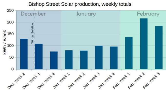
Bishop Street's 60 solar panels were installed on 12th Dec 2020, with a rated capacity of 20kW. The first ten weeks production are shown above and even in the gloomy days of January they produced 70kWh or more per week - equal to the typical weekly use in a UK home. A single sunny day in February was able to generate 50 kWh so we will be looking with interest at how they do over the summer. The graph below shows just how much UK electricity is now coming from carbon-free sources.
