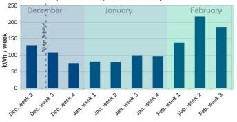
Bishop Street's 60 solar panels were installed on 12th Dec 2020, with a rated capacity of 20kW. The first ten weeks production are shown above and even in the gloomy days of January they produced 70kWh or more per week - equal to the typical weekly use in a UK home. A single sunny day in February was able to generate 50 kWh so we will be looking with interest at how they do over the summer. The graph below shows just how much UK electricity is now coming from carbon-free sources.
